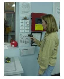
For capturing data, there are a variety of "dumb" devices, such as batch scanners, which capture and log data as a job is carried out. They record data both by time and by piece.
